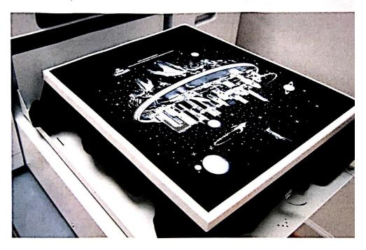
dark-polyester garment requires applying a light coat of polyester pretreatment, drying and repeating. The shirt can then be printed like normal. After printing, it should be heat set at 265°F for 45 seconds, cooled and cured twice. This technique may vary with specific garments and ink systems, so
